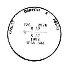
I used a steel tape and magnetic compass in the establishment of new accessories. I used 17° East magnetic declination and the distances are to a 50d spike driven in the right side of the root crown. I attached a brass washer marked OPLS 644 to the BT blaze.
