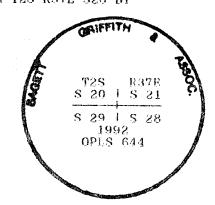
I used a steel tape and magnetic compass in the establishment of new accessories. I used 17° East magnetic declination and the distances are to a 50d spike driven in the right side of the root crown. I attached a brass washer marked OPLS 644 to the BT blaze.
