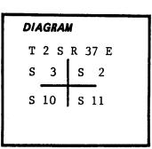
A pine 6 ins diam bears N 60° W, 8 1ks dist marked R 37 E S 3 BT. A pine 4 ins diam bears N 32° E, 50 1ks dist marked T 2 S S 2 BT. A pine 15 ins diam bears S 49° E, 15 1ks dist marked S 11 BT. A pine 5 ins diam bears S 34° W, 14 1ks dist marked S 10 BT.
