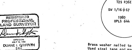
Brass washer nailed to B.T. blaze Used steel tape and magnetic compass with 20° East declination. Measured to center of all B.T.s
