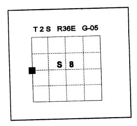
Found brass cap as per 239-84R marked as shown below. The SE bearing tree is alive and vigerous a 21" Pine with scribing visible. The NW bearing tree is The SE bearing tree is alive and vigerous a 26" White Fir with blaze evident.
