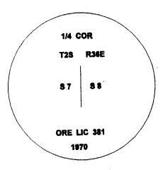
I used a steel tape and magnetic compass in the establishment of the new accessories. I used 18° East declination, the distances are to a 60d spike driven into the root crown of the bearing tree.
