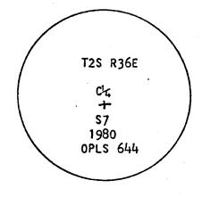
Brass washer nailed to B.T. blaze Used steel tape and magnetic compass with 20° East declination. Measured to center of all B.T.s
