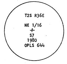
Brass washer nailed to B.T. blaze Used steel tape and magnetic compass with 20° East declination. Measured to center of all B.T.s
