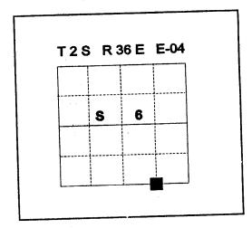
DESCRIPTION OF MONUMENT AND ACCESSORIES I ESTABLISHED At the position determined by the survey I set a 2½"x30" aluminum pipe with aluminum cap marked as shown, 12 inches in the ground with a mound of stones 3 feet base to top of cap, from which;
