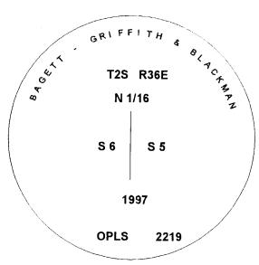
I used a total station instrument in the establishment of the new accessories. basis of bearing is the same as survey number 033-1997. The distances are to a 60d spike driven into the right side of the root crown of the bearing tree. I attached a brass washer marked OPLS 2219 to the BT blaze.
