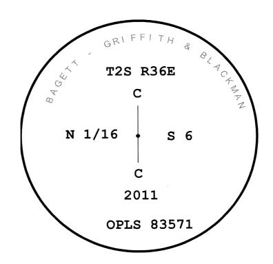
I used a magnetic compass and steel tape in the establishment of the accessories. Magnetic declination used was  $16^{\circ}$  East. The distances are to a 60d spike in the right hand side of the trees and bearings are to a brass washer marked OPLS 83571 to the center of the BT blaze.
