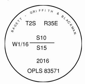
I use a steel tape and magnetic compass in the establishment of the accessories. Magnetic declination used was 15° East. Distances are to a 60d spike in the right hand side of the root crown of the bearing trees.
