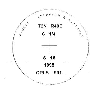
I used a steel tape and magnetic compass in the establishment of the new accessories. I used 17° East declination, The distances are to a 60d spike driven into the right side of the root crown of the new bearing trees. A brass washer marked OPLS 991 is attached to the BT blaze of the new trees.
