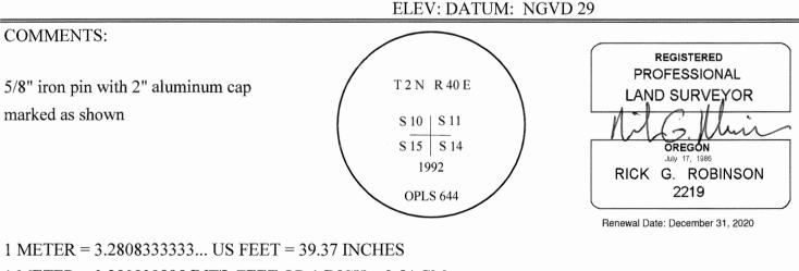
1 METER = 3.280839895 INT'L FEET OR 1 INCH = 2.54 CM TO CALCULATE ELEVATION FACTOR ( IN THE NORTH AMERICAN CONTINENT) DIVIDE 20,906,000 BY (20,906,000 + ELLIPSOID ELEV. IN FEET)
