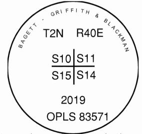
I used a steel tape and magnetic compass in the establishment of the new accessory. I used 13° East declination. Distances and bearings are to the center of the aluminum caps.
