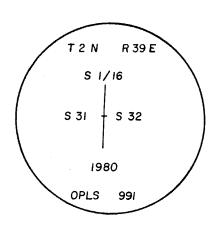
I used a steel tape and magnetic compass with 20° E declination. I set a brass washer marked OPLS 991 at the BT blazes.
