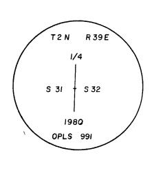
I used a steel tape and a magnetic compass with  $20^{\rm O}$  E declination. I set a brass washer marked OPLS 991 at the BT blaze.
