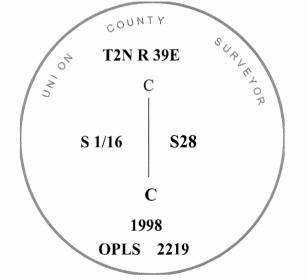
I used a steel tape and a magnetic compass in the establishment of the new accessories. I used 20° east magnetic declination. The distances are to a 60d spike driven into the root crown of the bearing tree. A brass washer marked OPLS 2219 is attached to the BT blaze.
