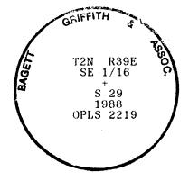
I used a steel tape and magnetic compass in the establishment of new corner accessories. I used 20° magnetic declination. The distances are to a 50d spike driven in the right side of the root crown. I attached a brass washer marked OPLS 2219 to the BT blaze.
