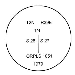
I used a steel tape and magnetic compass in the establishment of the new accessories. I used 16° East declination. The distances are to a 60d spike driven into the right side of the root crown of the bearing trees. A brass washer marked OPLS 83571 is attached to the BT blaze of the new bearing trees.
