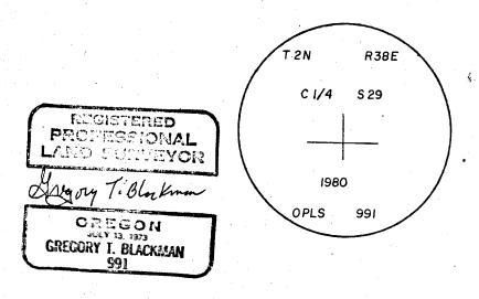
I used a steel tape and magnetic compass with  $20^{\circ}$  declination East declination. I set a brass washer marked OPLS 991 at the BT blaze.
