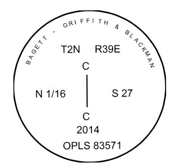
I used a steel tape and magnetic compass in the establishment of the accessories. I used  $16^{\circ}$  East declination. The distances are to a 60d spike driven into the right side of the root crown of the bearing trees. A brass washer marked OPLS 83571 is attached to the BT blaze of the bearing trees.
