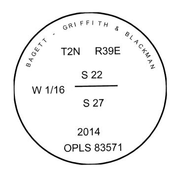
I used a steel tape and magnetic compass in the establishment of the accessories. I used 16° East declination. The distances are to a 60d spike driven into the right side of the root crown of the bearing trees. A brass washer marked OPLS 83571 is attached to the BT blaze of the bearing trees.
