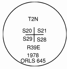
I used a steel tape and magnetic compass in the establishment of the new accessories. I used 13° East declination, the distances are to a 60d spike driven into the right side of the root crown of the bearing trees. A brass washer marked OPLS 83571 is attached to the BT blaze of the new bearing trees.
