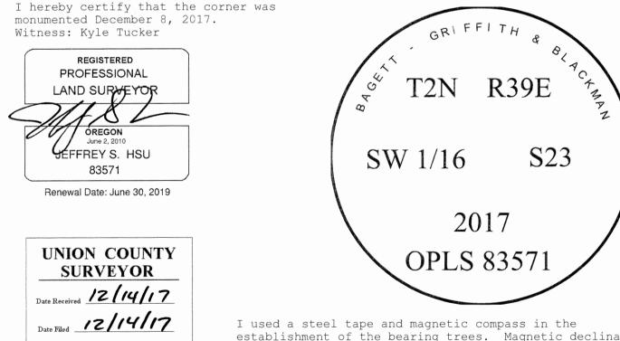
I used a steel tape and magnetic compass in the establishment of the bearing trees. Magnetic declination used was 13° East. Bearing is to a brass washer marked OPLS 83571 in the lower blaze of the tree. Distance is to a spike set in the root crown of the side of the tree.
