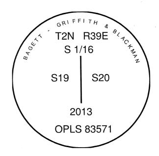
I used a steel tape and magnetic compass in the establishment of the accessories. I used 16° East declination, the distances are to a 60d spike driven into the right side of the root crown of the bearing trees. A brass washer marked OPLS 83571 is attached to the BT blaze of the new bearing tree.
