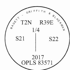
I used a steel tape and magnetic compass in the establishment of the bearing trees. Magnetic declination used was 13° East. Bearings are to a brass washer marked OPLS 83571 in the lower blaze of the tree. Distance is to a spike set in the root crown of the side of the tree.
