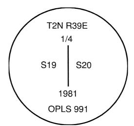
I used a steel tape and magnetic compass in the establishment of the accessories. I used 16° East declination, the distances are to a 60d spike driven into the right side of the root crown of the new bearing trees and to the center of the stump on the old. A brass washer marked OPLS 83571 is attached to the BT blaze of the new bearing tree.
