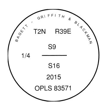
I used a steel tape and magnetic compass in the establishment of the new accessories. I used 15° East declination. The distances are to a 60d spike driven into the right side of the root crown of the bearing trees. A brass washer marked OPLS 83571 is attached to the BT blaze of the new bearing trees.
