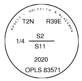
I used a steel tape and magnetic compass in the establishment of the new accessories. I used 14° East declination, the distances are to a 60d spike driven into the right side of the root crown of the bearing trees. A brass washer marked OPLS 83571 is attached to the BT blaze of the new bearing trees.
