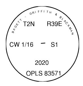
I used a steel tape and magnetic compass in the establishment of the new accessories. I used 14° East declination, the distances are to a 60d spike driven into the right side of the root crown of the bearing trees. A brass washer marked OPLS 83571 is attached to the BT blaze of the new bearing trees.
