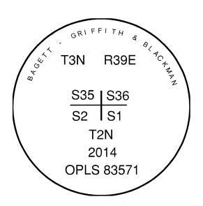
I used a steel tape and magnetic compass in the establishment of the new accessories. I used  $16^\circ$  Eas declination, the distances are to a 60d spike driven I used 16° East into the right side of the root crown of the new bearing trees. A brass washer marked OPLS 83571 is attached to the BT blaze of the new bearing trees.
