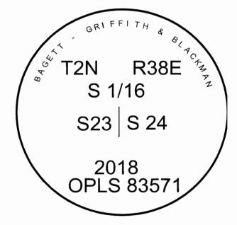
I use a steel tape and magnetic compass in the establishment of the bearing trees. Magnetic declination used was 13° East. Distances are to a spike in the root crown of the trees. Bearings are to a brass washer in the lower blaze marked OPLS 83571.
