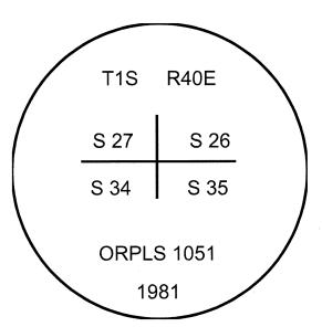
I used a steel tape and magnetic compass in the establishment of new accessories. I use a magnetic declination of 16° East. The distance to the bearing tree is to a 50d spike driven in the right side of the tree at the root crown. I attached a brass washer marked OPLS 83571 to the BT blaze.
