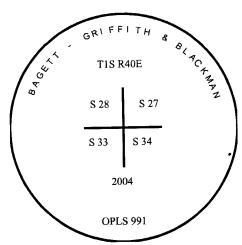
$\cI$  used a steel tape and magnetic compass in the establishment of the new accessories. I used 18° East declination. Distances are to a 50d spike driven into the root crown of the bearing tree in the right side. A brass washer marked OPLS 991 was attached to the BT blaze.
