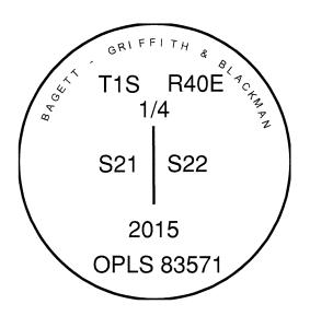
I used a steel tape and magnetic compass in the establishment of the new accessories. I used  $16^{\circ}$ East declination, the distances are to a 60d spike driven into the right side of the root crown of the bearing trees. A brass washer marked OPLS 83571 is attached to the BT blaze of the new bearing trees.
