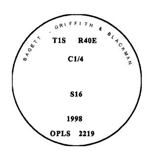
I used a total station instrument in the establishment of the new accessories. I used the same basis of bearing as survey number 043-1998, and the distances are to a 60d spike driven into the root crown of the bearing tree. A brass washer marked OPLS 2219 is attached to the BT blaze.
