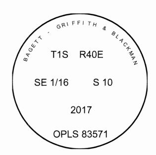
I used a steel tape and magnetic compass in the establishment of the bearing trees. Magnetic declination used was 13° East. Bearings are to a brass washer in the lower BT blaze marked OPLS 83751. Distances are to a spike in the side of the root crown.
