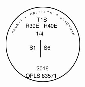
I use a RTK GPS unit in the establishment of the accessories. Basis of Bearings is as per Partition Plat for Kent Coppinger filed concurrently. Bearings and distances are to the center of the aluminum caps.
