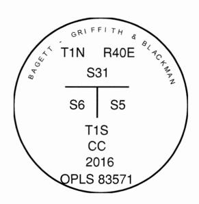
I use a RTK GPS unit in the establishment of the accessories. Basis of Bearings is as per Partition Plat for Kent Coppiner filed concurrently. Bearings and distances are to the center of the aluminum caps.
