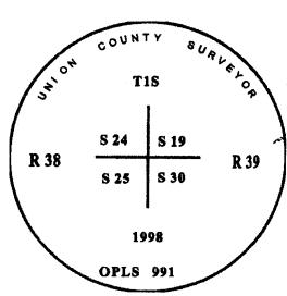
I used a steel tape and magnetic compass in the establishment of the new accessories. I used 17° East declination. The distances are to a 5/8"x30" rebar with 1 ½" aluminum cap marked Union county Survey Marker. In addition, the distances are two to existing 5/8" iron pins set by Voelz.
