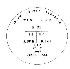
I used a steel tape and magnetic compass in the establishment of new accessories. I used 18° east declination and the measurement was taken to the center of the aluminum cap on the rebar.
