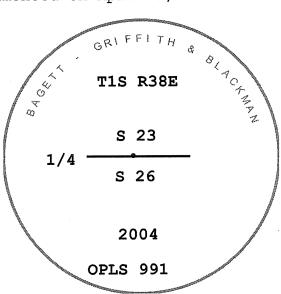
I used a Leica GPS-500 in the establishment of new accessories. The basis of bearings is the same as that on survey number 003-2004. The distances are to a punch in the center of the aluminum cap, the center of the wooden fence post.
