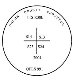
I used a GPS-500 receiver in the establishment of the new accessories. The basis of bearings is the same as that on survey number 003-2004. The distances are to the center of a 5/8" rebar with a 1 ½" aluminum cap. And 4" irrigation riser.
