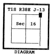
Survey 66-72 states finding a concrete monument at the corner position. Survey 137-78 states the concrete corner monument was gone and concrete reference monuments were used to place the corner position.
