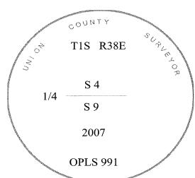
I used a steel tape and magnetic compass to establish the new accessories. I used 18° East magnetic declination. The distances to the pins are to the center of the aluminum cap.
