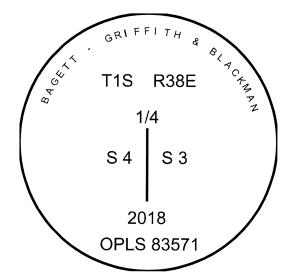
I used a RTK GPS in the establishment of the accessories. Basis of bearing is as per Survey Number 036-2018. Bearings and distances are to the center of the aluminum caps.
