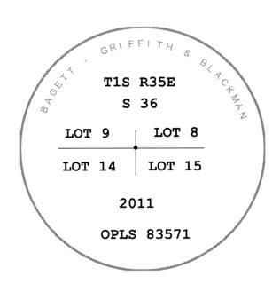
I used a magnetic compass and steel tape in the establishment of the accessories. Magnetic declination used was 16° East. The distances are to a 60d spike in the right hand side of the trees and bearings are to a brass washer marked OPLS 83571 in the upper portion of the BT blaze.
