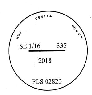
I use a tape and compass in the verification of the existing bearing objects. 14° East was used for declination and measured to a brass washer labeled "OPLS 02820" in the BT blaze at the base of the tree. Distances are to a 60D nail in the right wide of the base of the center of the tree.
