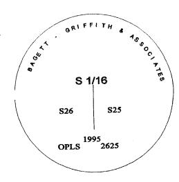
I used a steel tape and magnetic compass in the establishment of the new accessories. I used 18° East declination, the distances are to a 50d spike driven in the right side of the root crown. I attached a brass washer marked OPLS 2625 to the bearing tree blaze.
