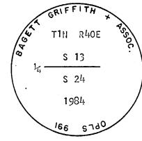
I used a steel tape and magnetic compass in the establishment of accessories. I used 18° East magnetic declination, and distances to the new BTs are to the center of the tree. I placed a brass washer marked OPLS 991 by the BT blaze of new BTs.
