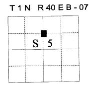
A 5/8" x 30" rebar with plastic cap bears S19°E, a distance of 92.88 feet, marked "BGB SURVEY MARKER". A 5/8" x 30" rebar with aluminum cap bears N46°W, a distance of 32.93 feet, marked "NW RP".
